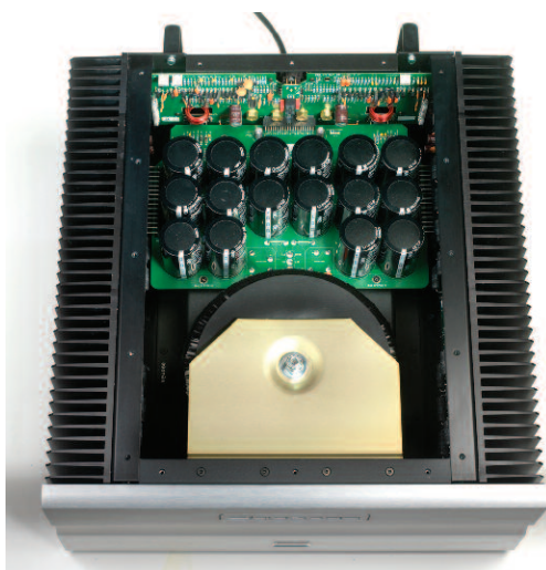
The 28B-SST's interior is dominated by the enormous toroidal transformer.
