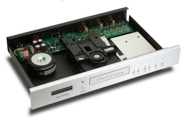
Speaking of which, the engineers at Bryston have chosen the same DAC for the BCD-1 that they already use in the company's preamps and integrated amps: the Crystal CS4398. The chip first upsamples the incoming signal from 44.1kHz to 192kHz and then oversamples it 128 times to create a new sampling frequency before running it through an interpolation filter
