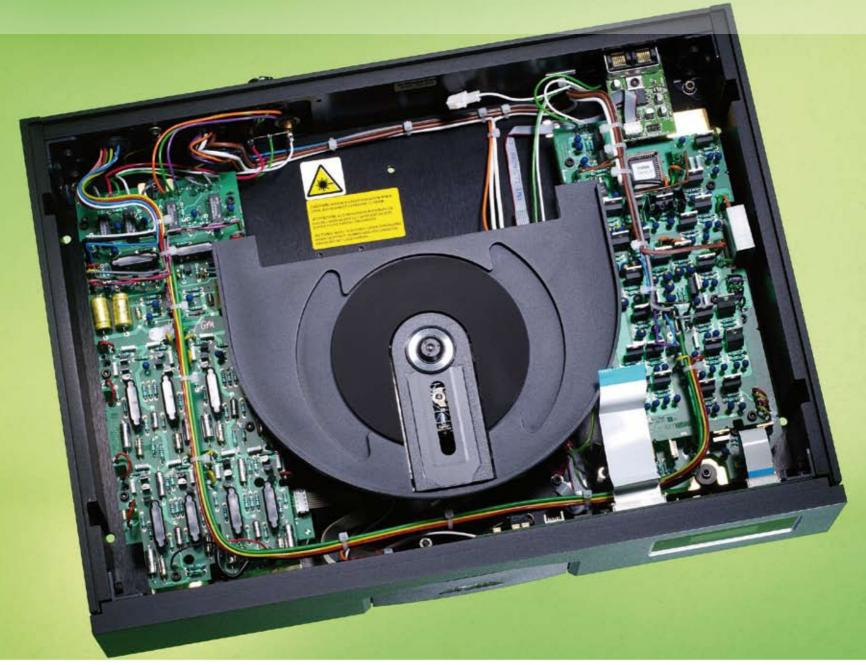
Clean spatial division: The picture above shows the digital section (left) mounted using SMD technology (links) and the conventionally equipped analog circuit board (right). Below: the casing top turned inside out with the driver cover and the motorization.
