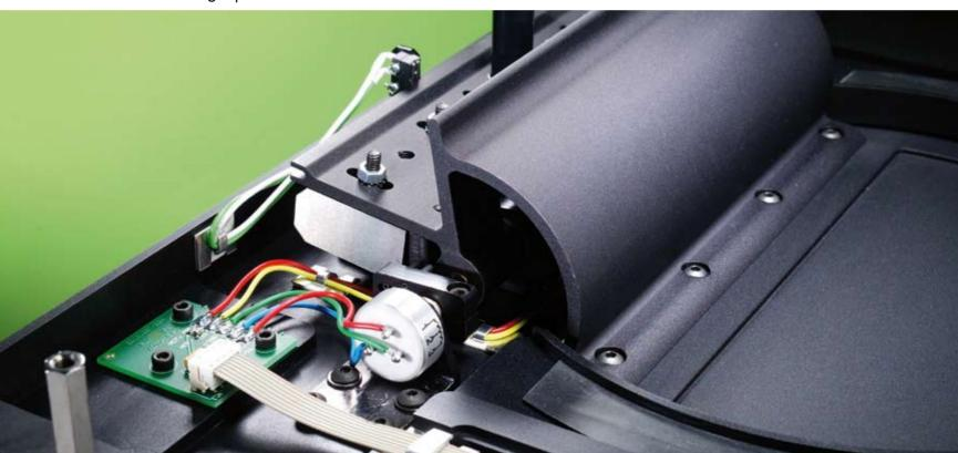
mechanical and electrical vibrations. Shock absorbers - pins in jacket on leaf springs - are meant to prevent this. They suspend the circuit boards responsible for processing digital and analog signals in a decoupled position. The springs for the drive and the circuit boards are adjusted differently in accordance with the signal properties.
