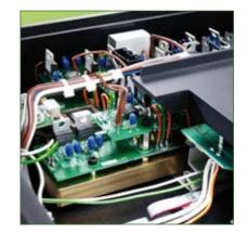
With clean signals of this sort the converter chip finds it easy to separate the control from the music signal. The latter is produced by an ultra-precise pulse generator directly in front of the converters. Naim has partitioned the quartz with triple regulated voltage and its own filters completely from the player electronics.
