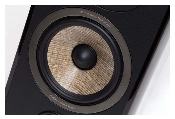
Although flax represents less than 1% of the fibers used in textiles, France is the world's biggest producer of flax. That makes it a natural fit for Focal, which is based in La Talaudière, France. Focal found that the hollow-cored flax fibers have half the weight of glass fiber but very low elasticity. It proved to be an ideal core material -- and with a sheet of glass fiber on either side of a flax core, the F sandwich was born. According to Focal, this composite material has high
