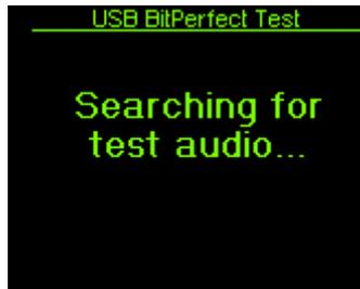
As the audio file progresses, the DAC-V1 will update the display to indicate how far through the test file it is, if any errors are found then they will be shown on this display.
